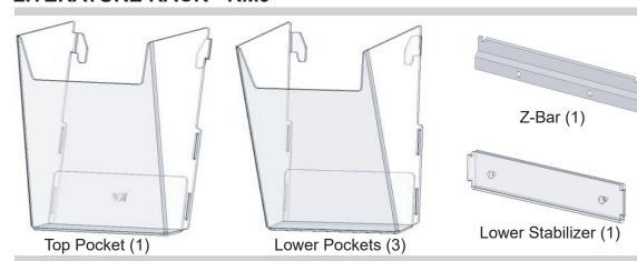
1. Place z-bar in desired location on a wall and mark the holes using a pencil. Remove z-bar and drill two 7/32" holes. Insert anchors and attach z-bar with screws.
