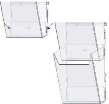
4. After installing last pocket, make two line marks on the wall at the bottom of slots (see images below), then remove last pocket. Align stabilizer to marks and mark the holes on the wall. Drill two 7/32" holes, install stabilizer using anchors and screws provided. Reinstall last pocket and attach tabs into the slots on the last pocket.
